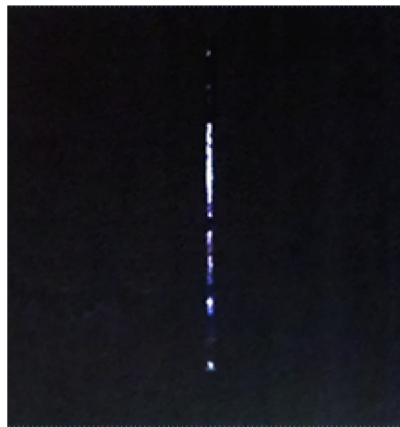
Figure 3: Photo of thermal image of a crack obtained in 2-3 seconds (light areas)
