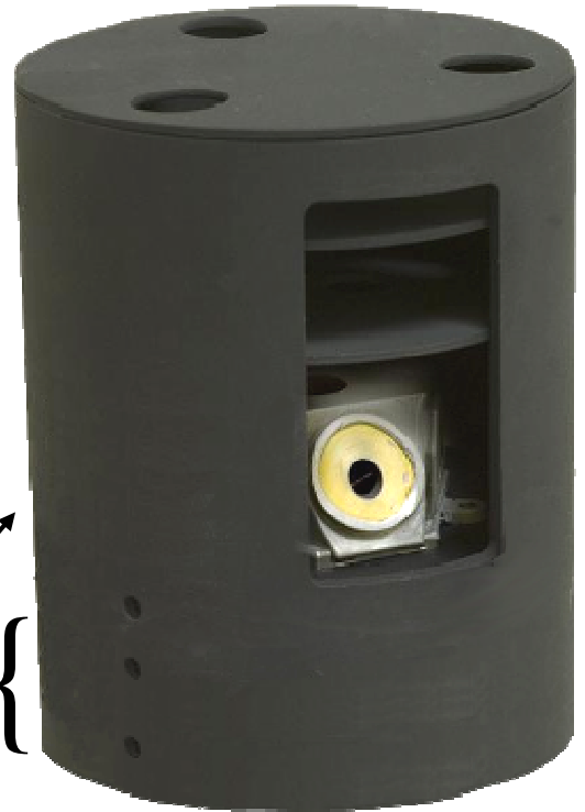
MDE1300 Star Tracker fully integrated with space computer and power supply
